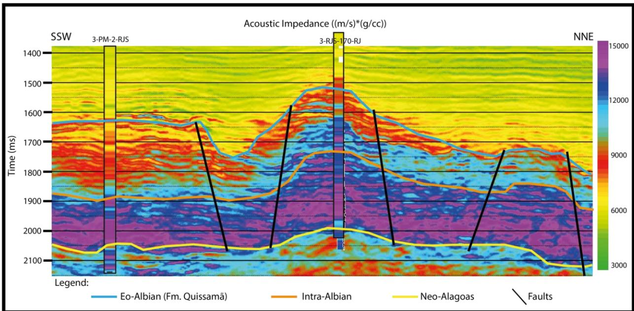
**Figure 6:** Acoustic impedance values in the arbitrary line 1. The Eo-Albian, Intra-Albian and Neo-Alagoas seismic horizons are represented, respectively, by the lines in blue, orange and yellow. Faults are represented in black lines. The acoustic impedance logs of the 3-PM-2-RJS and 3-RJS-170-RJ wells are also shown.
