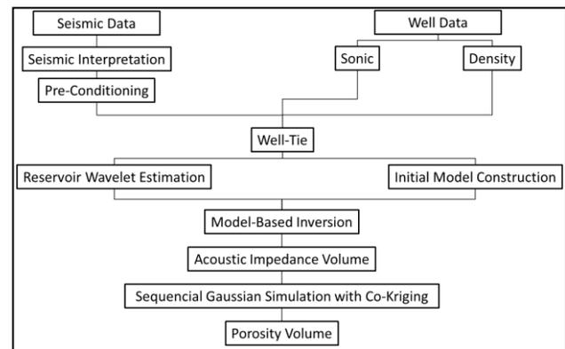
**Figure 3:** Workflow used to characterize the carbonate reservoirs of Pampo Field.
