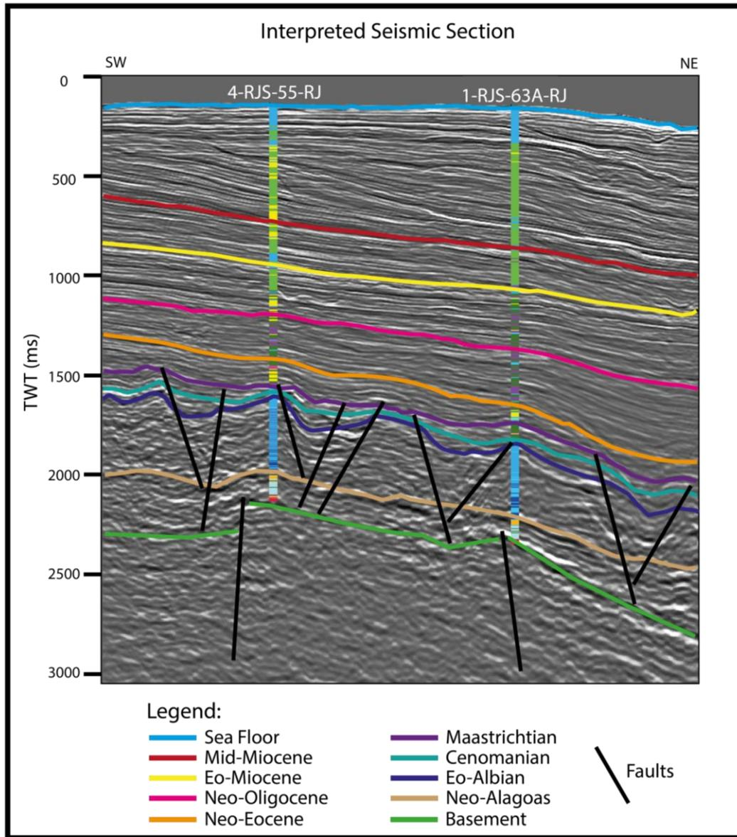
**Figure 4:** Seismic Interpretation in the Inline 1260.
