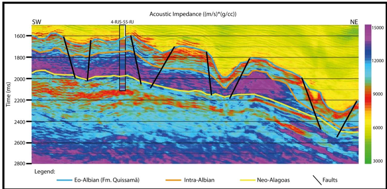
**Figure 5:** Acoustic impedance values (inline 1260). The Eo-Albian, Intra-Albian and Neo-Alagoas seismic horizons are represented, respectively, by the lines in blue, orange and yellow. Faults are represented in black lines. The acoustic impedance logs of well 4-RJS-55-RJ can also be observed.
