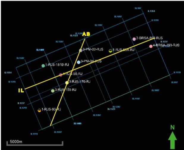
**Figure 2:** Data available for the study. The seismic cube survey is represented by the blue polygon, the wells are represented by colored circles and the acoustic impedance sections shown in Figures 5 and 6 are the yellow lines IL and AB, representing the inline 1260 and an arbitrary line respectively.
