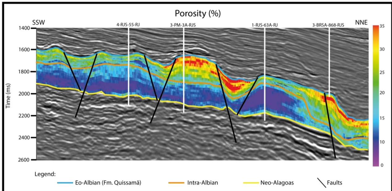
Figure 8: Porosity modelling in inline 1279. The Lower Albian, Intra-Albian and Upper Alagoas seismic horizons are represented, respectively, by the lines in blue, orange and yellow. Faults are represented in black lines. The well path of the wells that intersect or are located near the inline can also be observed.
